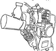
Neither overfill nor spill the fuel on to the engine.
