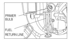
STEP #4) Pump the "PRIMER BULB" under of the carburetor until fuel can be seen flowing through the "FUEL-RETURN LINE".
