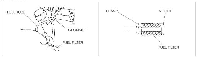
To clean the fuel filter, remove it from the fuel tube and wash it with safety solvent. Inspect and clean the fuel tank before re-installing the fuel filter.
