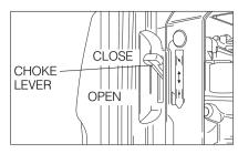
STEP #5) Move the "CHOKE LEVER" fully up ward to the closed position. If the engine is already warm, only a partial or open (no choke) choke setting may be required.
