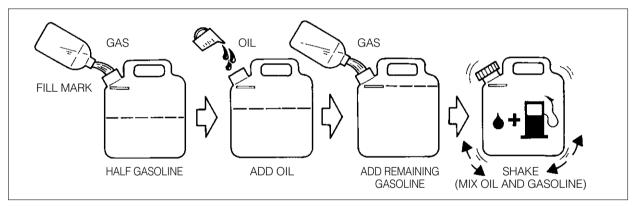
momentarily to evenly mix the oil and the gasoline before filling the fuel tank on the product. When refilling the fuel tank, clean around the fuel tank cap to prevent dirt and debris for entering the tank during cap removal. Always shake the premix fuel container momentarily before filling the fuel tank.
